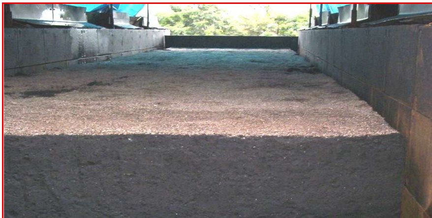
COATED COMPACTED COAL CAKE READY FOR CHARGING INTO THE OVEN
