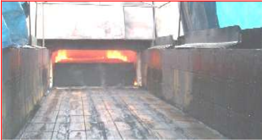
COATED CAKE PUSHED INTO OVEN (NOTE FLAMES AT SIDE ONLY)
