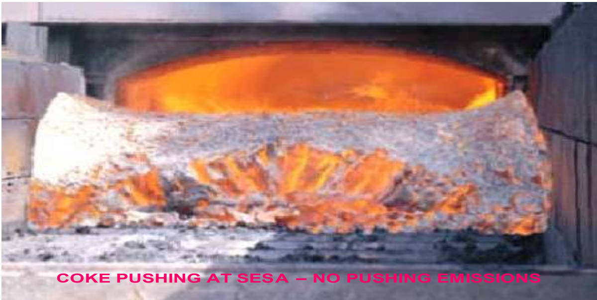
COKE BEING PUSHED INTO THE QUENCH CAR – NO PUSHING EMISSIONS
